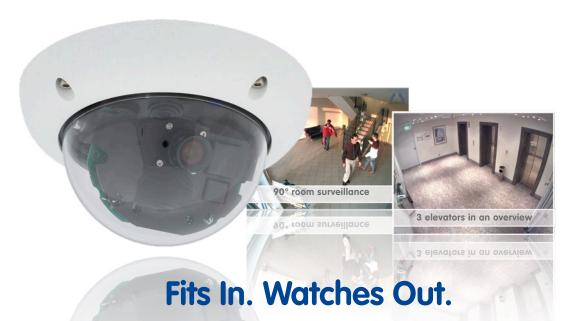
Inconspicuous surveillance with state-of-the-art technology. The D24 FixDome from MOBOTIX adapts perfectly to any task. Exchangeable lenses, various mounting and configuration options including vandalism set support unlimited application possibilities.
