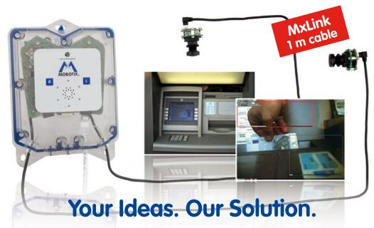
M12 DevKit is the ideal solution for all non-standard applications. It is a high-resolution dual IP camera with two separate image sensors that has been designed specifically for customized, concealed installations. With the M12 DevKit, there are no limits to your ideas.
